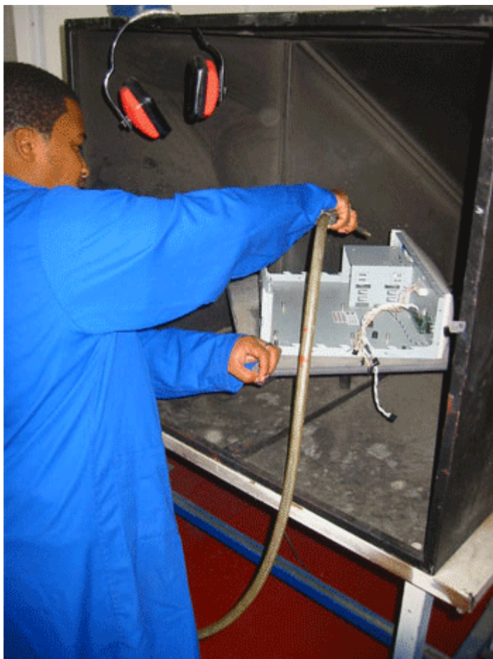
A technician uses the rotatable tray to clean a case before inserting a motherboard.
